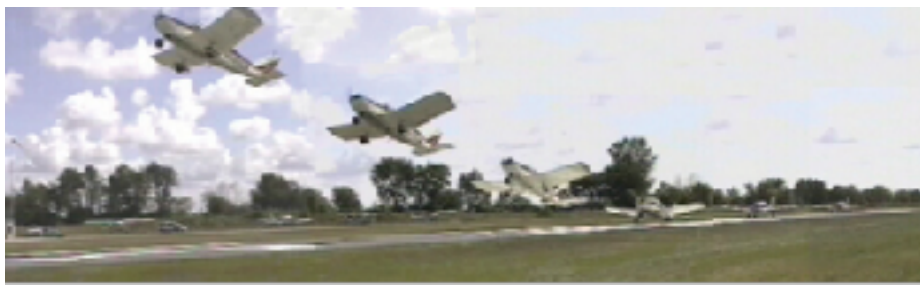
Above: Do not climb away like a Boeing, rather let the speed build before you start to climb at best rate or angle
