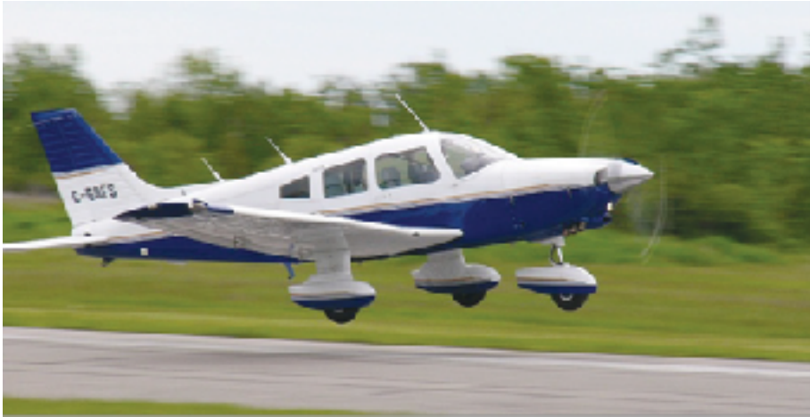
Above: Level off immediately after liftoff and accelerate in ground-effect until you have climb speed
