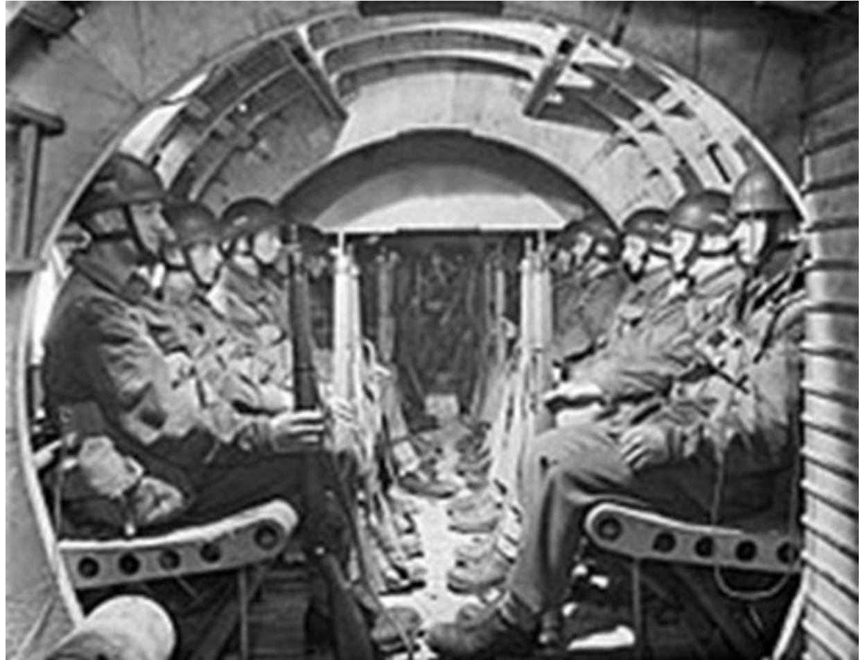
View inside the fuselage of a Horsa Glider. Troops were not strapped in & motorcycles were often carried down the centre between the soldiers.
